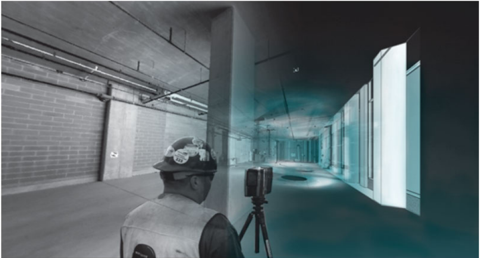
2.19 Composite image of a photo and model data (courtesy of Mortenson Construction).
